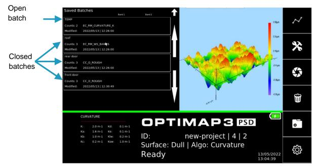
Until the latest batch is closed, from the project menu, the batch name is "TEMP".
