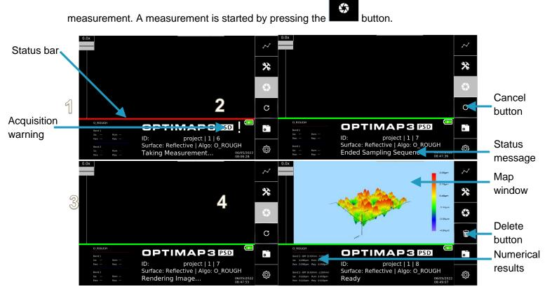
1. When the measurement button is pressed it will grey out to show that the instrument is taking a measurement. The status bar will turn red and acquisition warning (!) will show to illustrate that the instrument should not be moved while acquiring images, to be used in the calculation. The status message will show that the instrument is in the "Taking Measurement" part of the process. The only button that is active during the measurement process is the cancel
