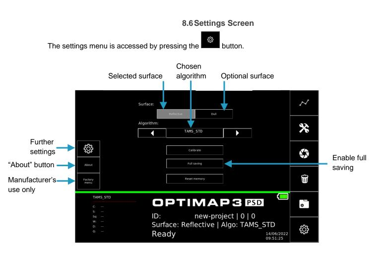
To allow the measurement of a wide range of surface finishes the Optimap has two optical configurations (models) available for selection – Reflective and Dull.
