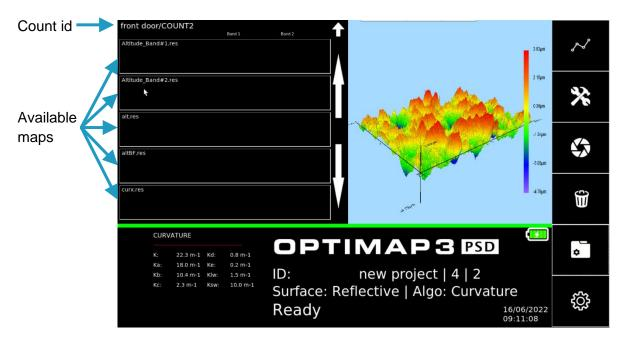
The available maps will depend on the algorithm and saving options. As count 0 is the average of the calculated parameters it contains no maps. Maps can be reviewed by pressing the entry. The rendering process can take some time, with no indication to show progress.
