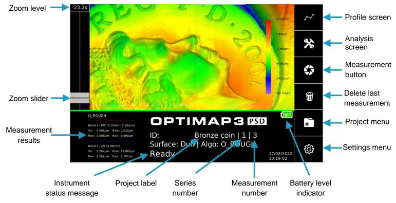
The touch sensitive icon-based measurement screen provides operation and setup of the device.
