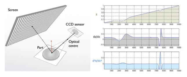
By differentiating the slope information curvature data can be produced allowing accurate characterisation of the surface profile.
