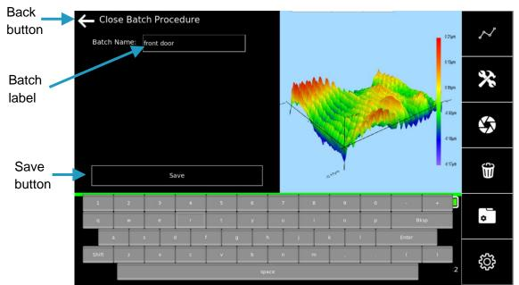
The desired name is entered using the on-screen keyboard, removing the default name of the batch number if not wanted using the "bksp" key and entering the desired name and completed by pressing the save button. Each batch within a project must have a unique name.
