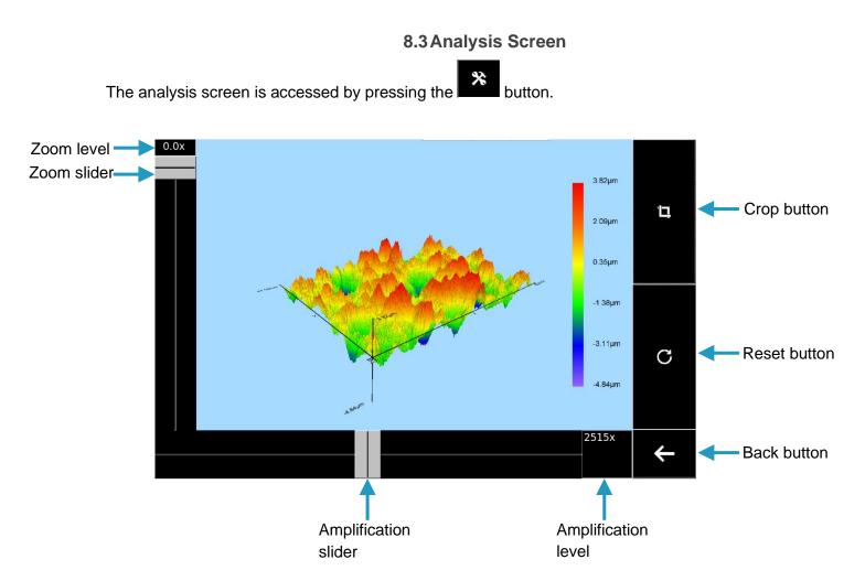
The analysis screen is used to interact with the map in more ways than the main screen allows. These include a larger window, moving and rotating the map, changing the zoom level, changing the amplification level, changing crop values, and resetting to default settings.
