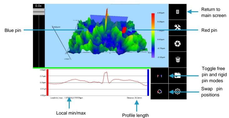
The profile has two modes; either the pins can be moved independently anywhere on the map, or the length of the profile and relative positions of the pins is fixed, and the
